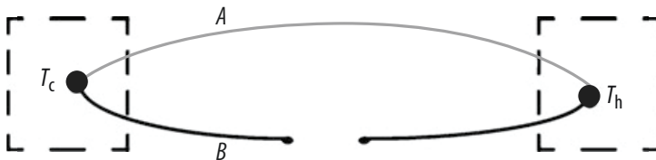
■ Fig. 9.1 Thermocouple basic circuit
